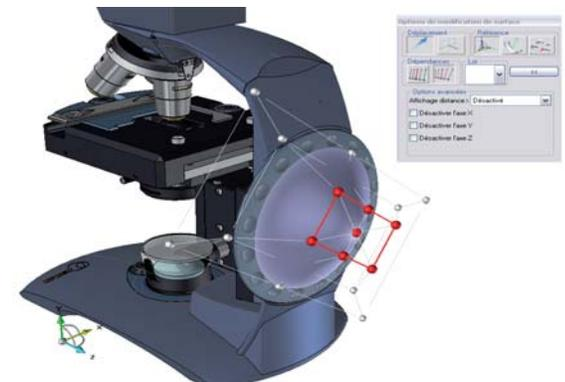
Modification of control points with TopSolid'Design.
